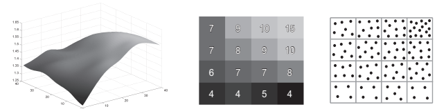
Figure 12: Blending the sampling rate at the patch boundary. Left: Continuous sampling rate. Middle: Discretized area weighted sampling rate. Right: Resulting sampling pattern.
